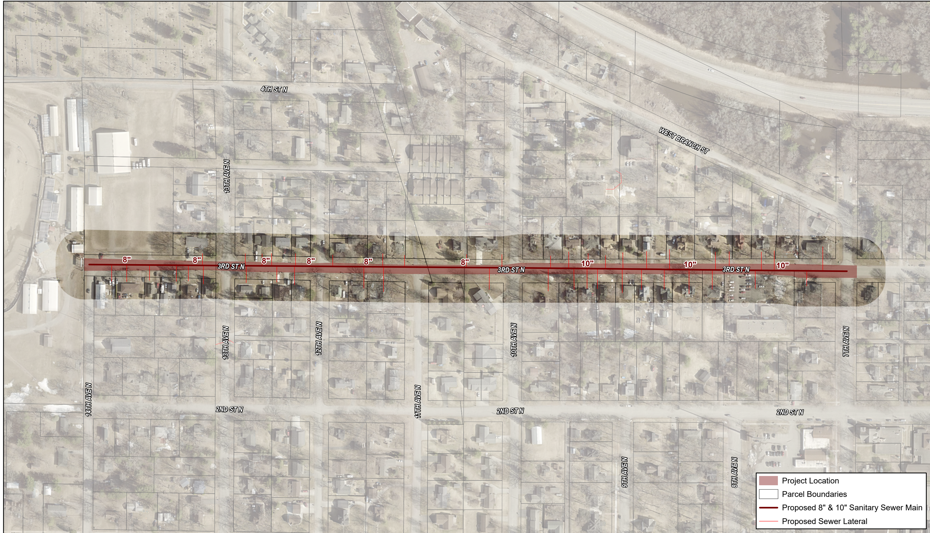
Figure 3B - Proposed Sanitary Sewer
