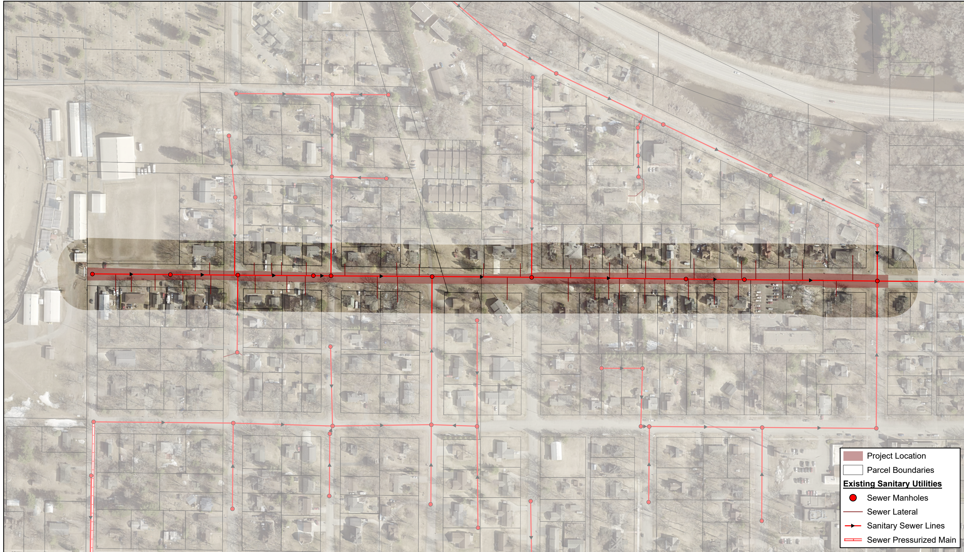
Figure 2B - Existing Sanitary Sewer
