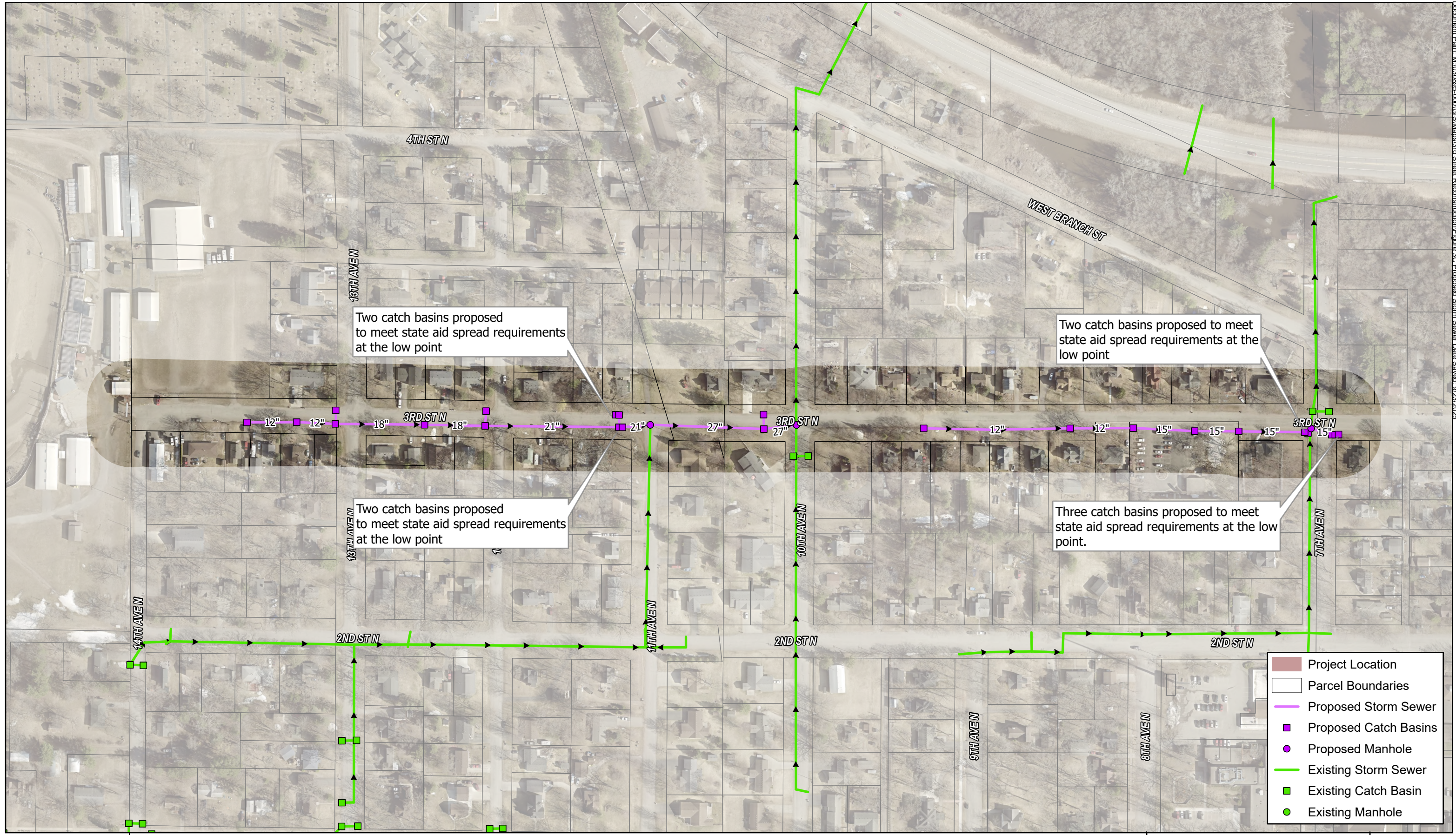
Figure 3C - Proposed Storm Sewer
